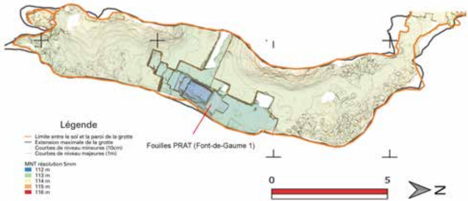
Figure 5: Topographical reconstruction of the Prat gallery, Get in Situ (X. Muth) based on laser-grammetric surveys carried out by Perazio Engineering.
